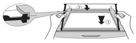
**3.** Lower the middle pane of glass (2) and slide it under the lower bracket to the stop.
